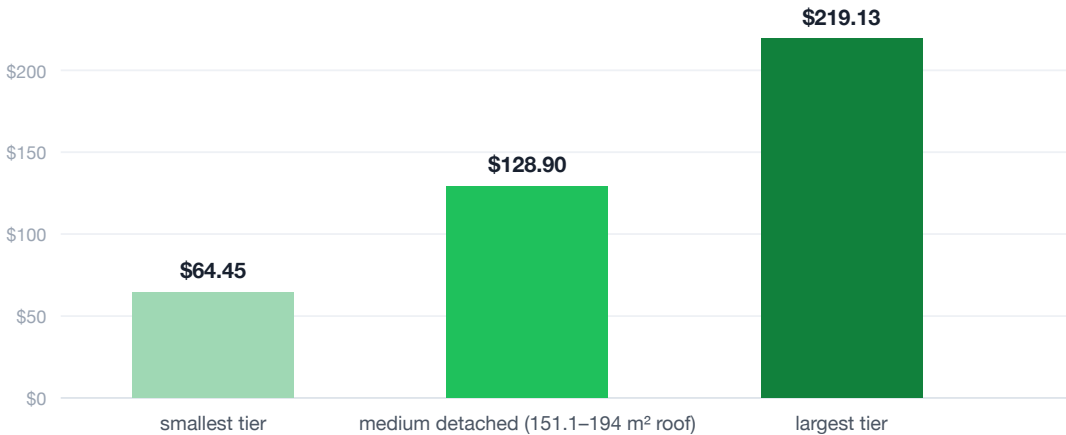
Figure 2 — Mississauga's 2026 stormwater charge: five rooftop-area tiers span $64.45–$219.13/yr (smallest, medium and largest shown). The charge keys to rooftop area, so lawn-surface choice does not change it. Source: City of Mississauga stormwater charge page [7].
